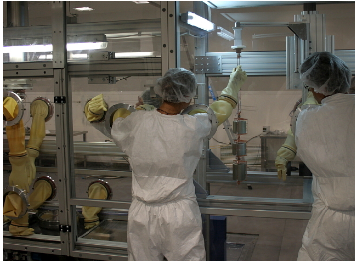
Figure 4.3: The first string deployed in GERDA during mounting in the glove box.
