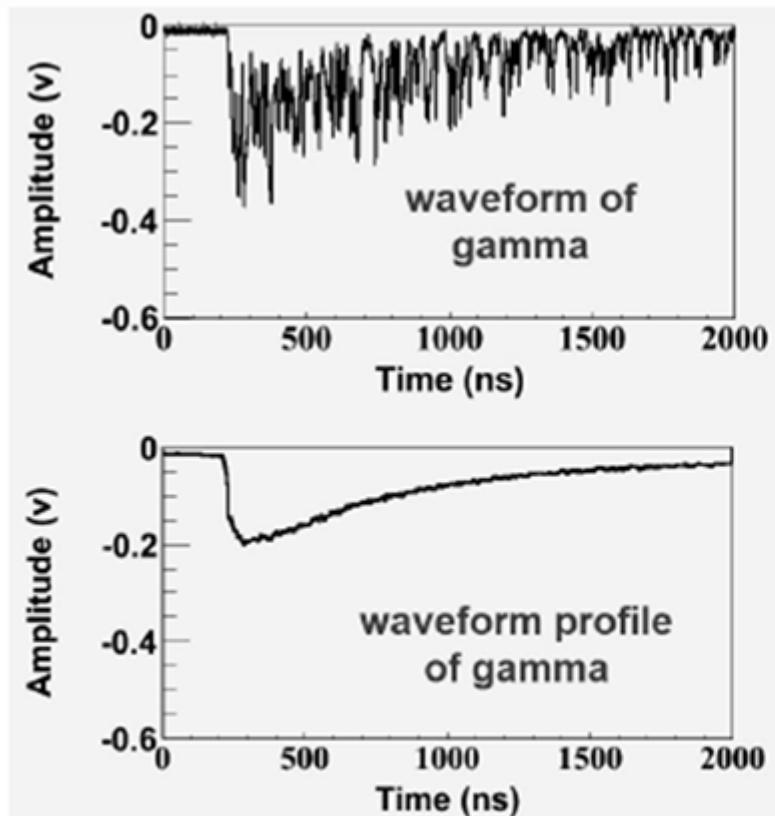
Fig. 7 A typical waveform of pure  $\gamma$ -ray (59.5 keVee) from (50-60 keVee).
