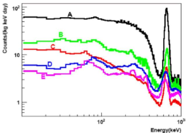
Fig. 6. Background spectra of various crystals; A: Best crystal in the market, B: Crystal was made by careful powder selection, C: Crystal was made by powder with "pure" water, D: Crystal was made by powder with recrystallization and "pure" water, E: Crystal was made by powder with recrystallization and "ultrapure" water.
