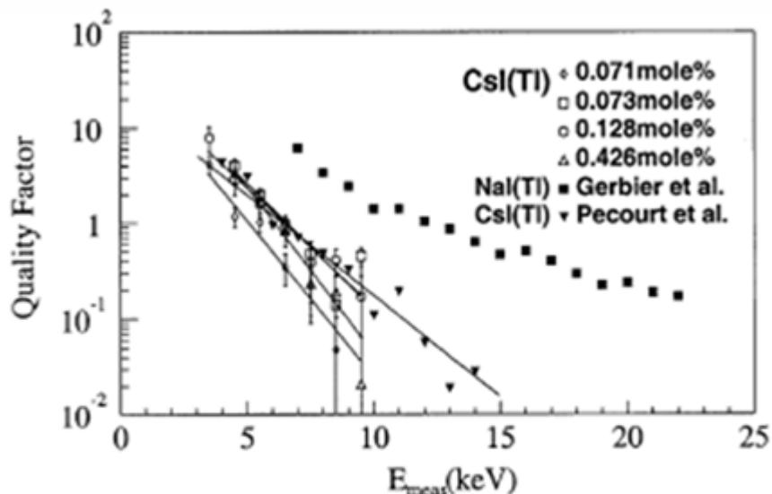
Fig. 10. Quality factors for various CsI(Tl). The errors are only statistical. The present results (open markers) are compared to the data of Pécourt et al. [10] and of Gerbier et al. [19].
