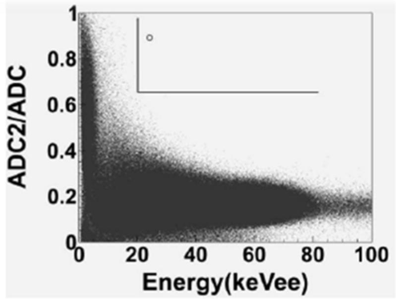
Fig. 10. Scatter plot of ADC2/ADC as a function of energy for  $\gamma$ -ray events. Only one event (in the small round circle) was seen in the region of  $\text{ADC2}/\text{ADC} > 0.65$  and energy  $> 20 \text{ keVee}$ .
