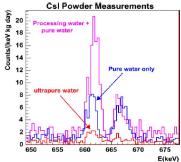
Fig. 5. The measured spectra of three different CsI powder samples with the HPGe detector. The peak near 665 keV is caused by gs from  $^{132}\text{Cs}$  and  $^{126}\text{I}$ .
