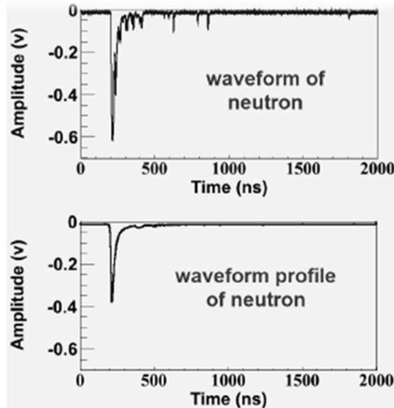
Fig. 8 A typical waveform of neutron (10 keVee) from (5-10 keVee).
