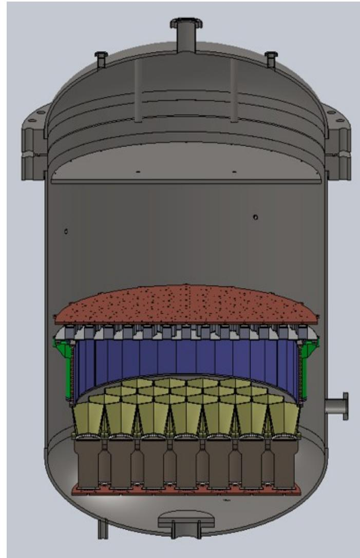
Passive shielding with Cu, Pb and PE
