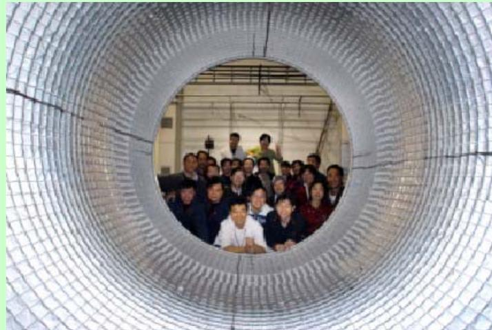
**Calorimeter to measure energy**
