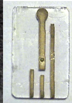
JFET bonding on silica substrate
