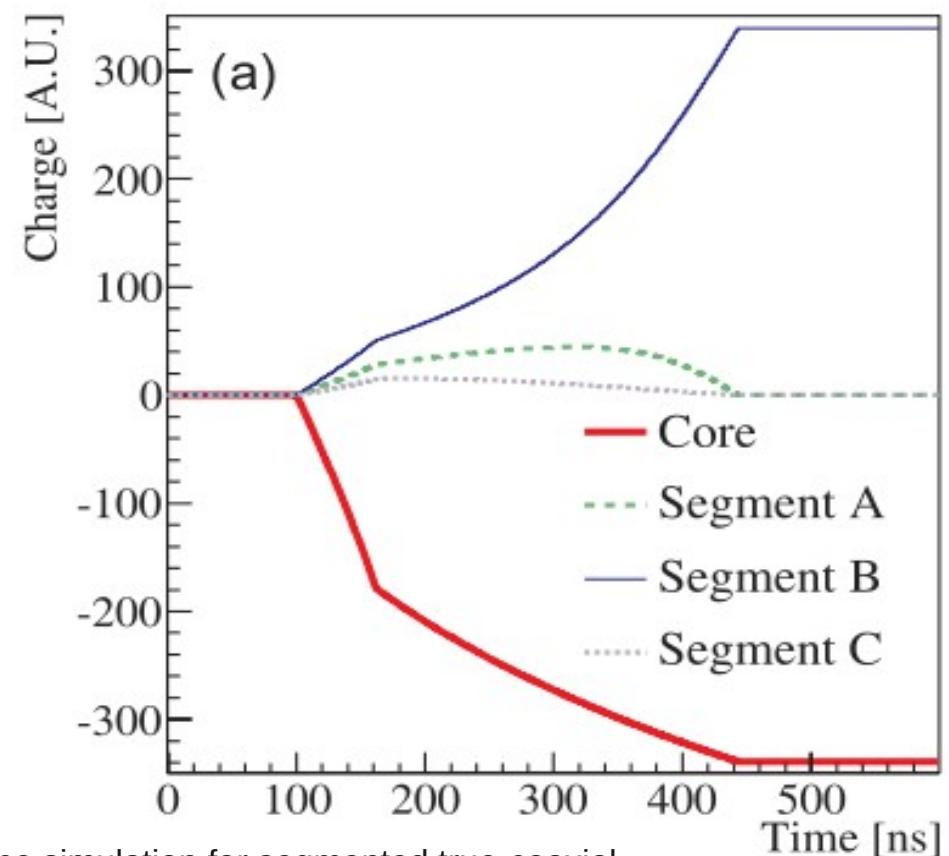
**Mirror Pulse:** charge „trajectory“ does not end at considered segment electrode
